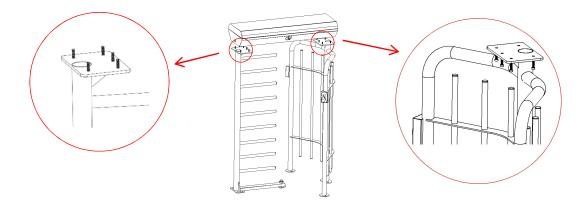
7. Put the whole rotating part in the middle of the frame and chassis and then fix up with screw and connection block.
