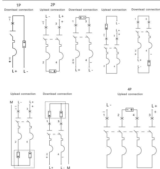
5.6 Wiring: Apply to 25 mm<sup>2</sup> wire connection terminals
